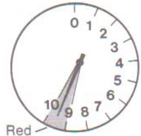
(c) Sector Target Zone (Can be read about 85% faster than the dial in a and is easier to interpret)
