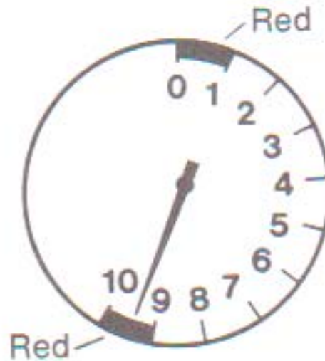
(b) Perimeter Target Zone (Can be read about 25% faster than the dial in a)
