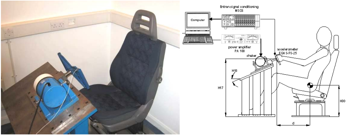
[Figure 1] Steering wheel vibration test rig and associated electronics used in the test experiment.
