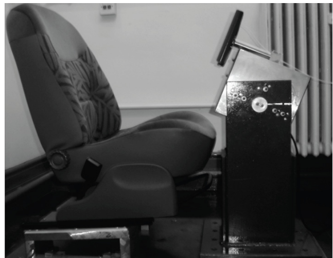
Figure 6: Steering wheel vertical vibration test facility.
