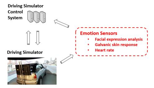
Figure 1 – Emotion-augmented driving simulator high-level architecture.
