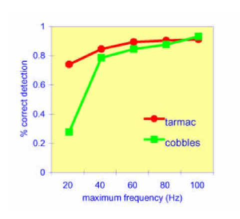
Figure 5 Percent correct detection results from the experiment to investigate the effect of stimuli frequency bandwidth.
