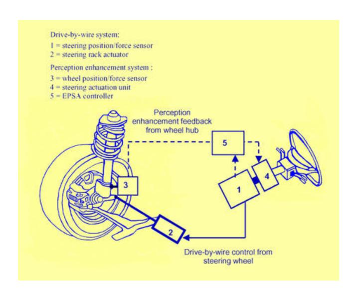
Figure 1 A perception enhancement system for by-wire steering.
