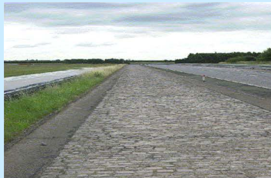
Cobblestones road (vehicle speed : 30kph)
