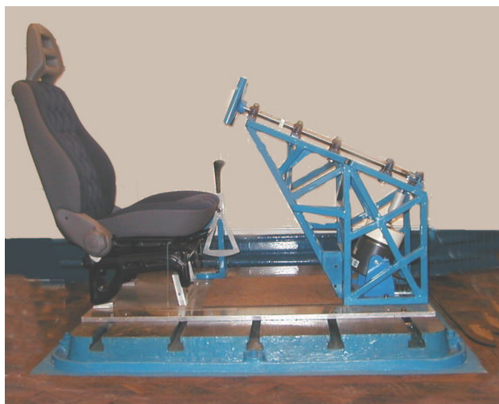
Figure 2) Steering wheel rotational vibration test bench
