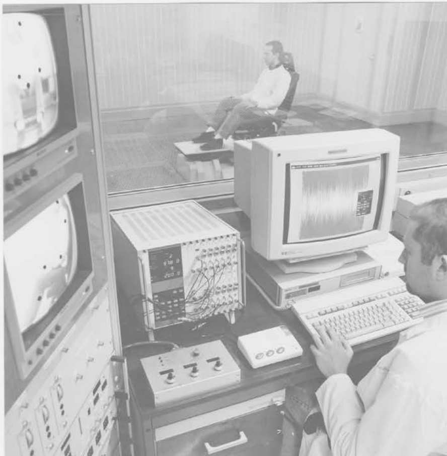
Figure 4) CRF Seat testing cell.
