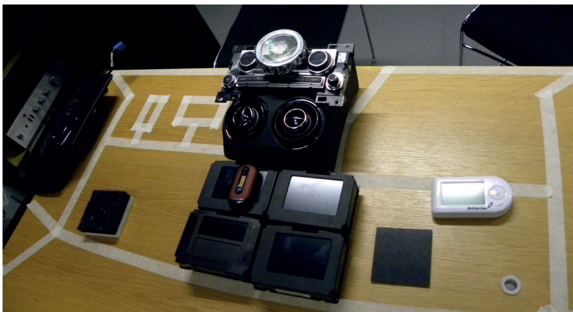
Fig. 3 An example 'natural feeling dashboard' creation, showing a 'sparse' layout focused around the driver, with dark and matt materials
