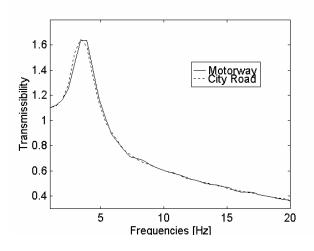
Figure 6) Transmissibility function from the floor to mass  $m_1$  for the motorway and for the city road acceleration inputs.
