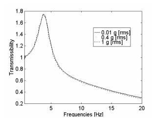
Figure 4) Transmissibility function from the floor to mass  $m_1$  for various levels of random white noise acceleration input.
