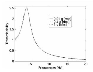
Figure 5) Transmissibility function from the floor to the upper mass m<sub>nonlinear</sub> for various levels of random white noise acceleration input.
