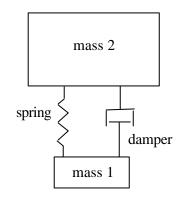
Figure 2) Lumped parameter model of the human body from reference 10.
