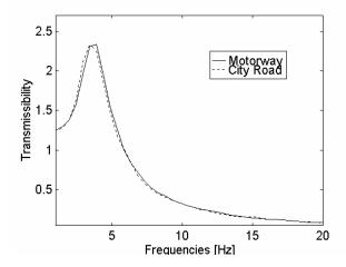
Figure 7) Transmissibility function from the floor to  $m_{nonlinear}$  for the motorway and for the city road acceleration inputs.
