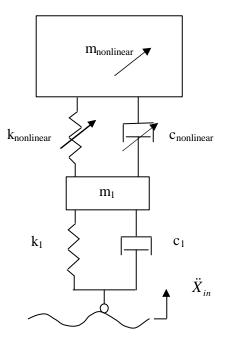
Figure 3) Nonlinear lumped parameter model of the person/seat system.
