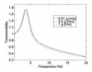
Figure 8) Transmissibility function from floor to mass  $m_1$  for the seat cushion with added cubic stiffness term.
