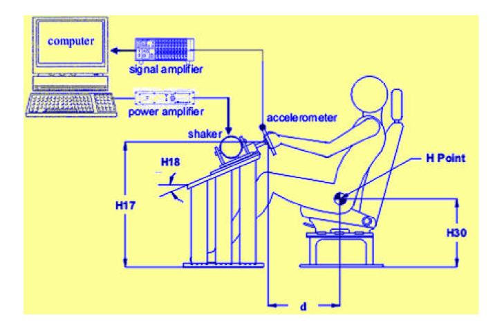
Figure 6 Steering wheel rotational vibration test simulator.
