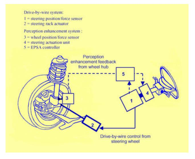
Figure 2 A perception enhancement system for by-wire steering.
