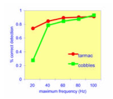
Figure 8 Percent correct detection results from the experiment to investigate the effect of vibration frequency bandwidth.
