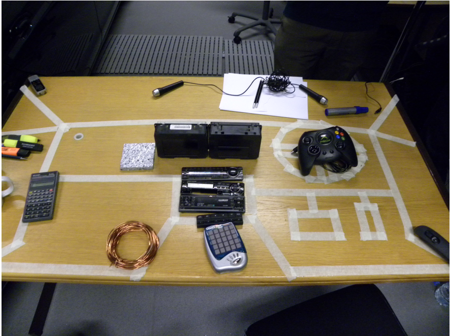
Figure 8: An example ‘unnatural feeling dashboard’ creation, exhibiting many small identical buttons, rough and metallic textures, and sources of visual distraction.
